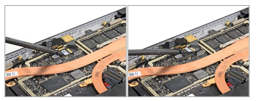
Use the flat end of a spudger to pry up on the rear camera connector and disconnect it from the motherboard.
