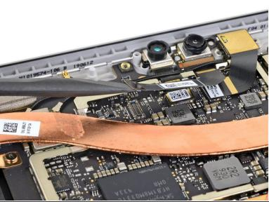
Use the flat end of a spudger to pry up the Hello face camera connector and disconnect it from the motherboard.
