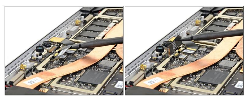
Use the flat end of a spudger to lift the front camera ribbon cable off of the rear camera connector.
