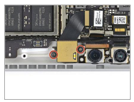
Use a T3 Torx screwdriver to remove the two 2.6 mm screws securing the rear camera to the case.
