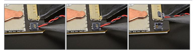
Use the pointed end of a spudger to lift and disconnect the right speaker wire from its connector on the motherboard.
