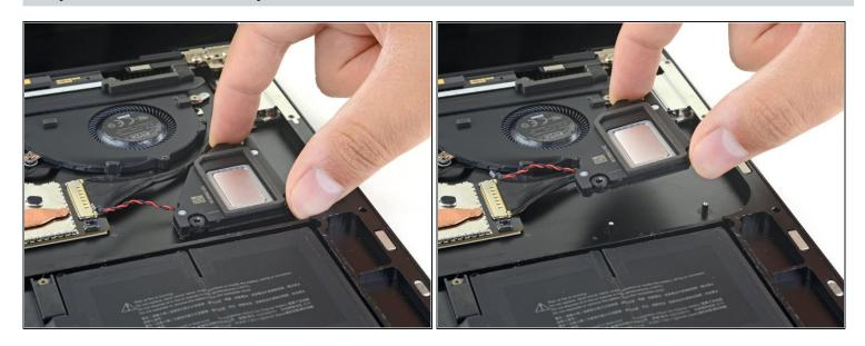
Lift and remove the right speaker from its three posts.
