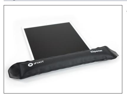
• Use your <u>iOpener</u> or hair dryer for about a minute to heat the home button area in order to soften the adhesive securing the home button components.
