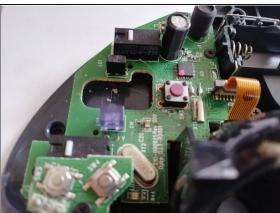
• After the screws are loosened, the housing can be easily removed. The space for the blue ball is made of its own piece of plastic. The circuit board is held in place with a few screws.
