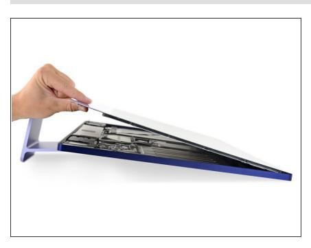
After the adhesive has been removed, you can use a suction cup to help remove the display from the case.
