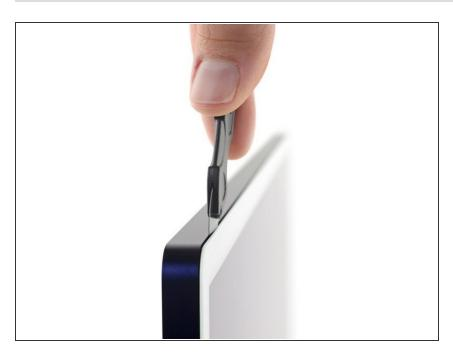
Start by gently peeling the adhesive off of each side of the iMac by using the iMac Opening Wheel.
