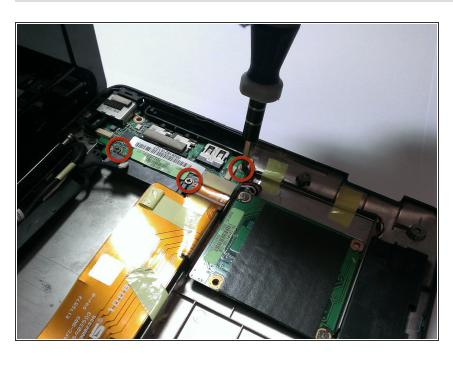
USB header card: Use the Phillips head screwdriver to unscrew the 3 screws from the USB header card.
