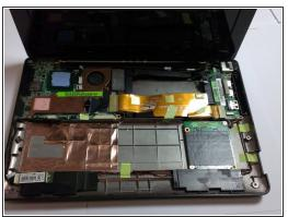
Battery: Use your fingers to lift the battery and gently disconnect the wires from the base.
