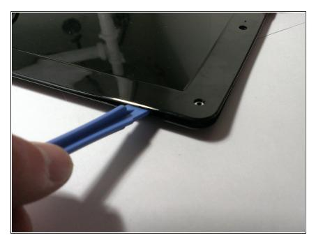
Slide the Plastic Opening Tool under the edge of the screen bezel to release the front panel of the screen.
