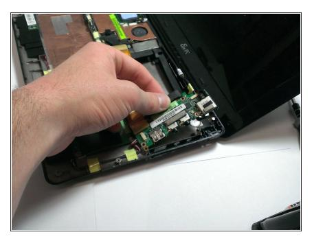
Use your fingers to pull the USB header card from the side of the device chassis. (The USB header card will remain attached by wires.)
