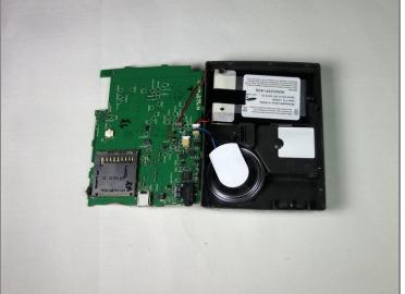
• The motherboard will now freely separate from the back casing; lay it flat next to the housing.
