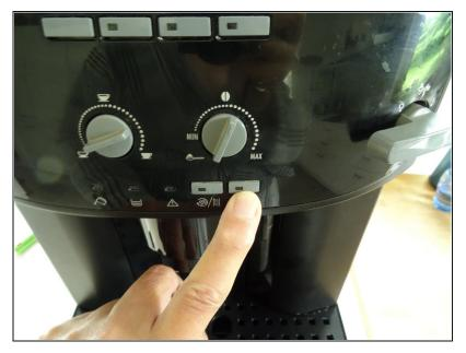
• Press the "ECO" key. The grinder should be activated.
