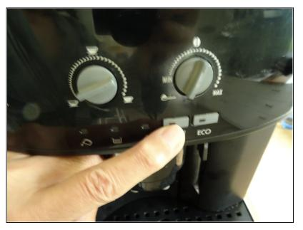
Press the "Rinse" key. One LED should light up and the heater should be activated. If it reaches the end temperature, the LED goes out.
