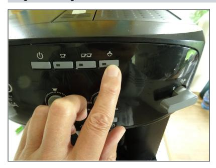
Press the "steam" key. The pump should be activated. If the steam wand is opened the water should flow.
