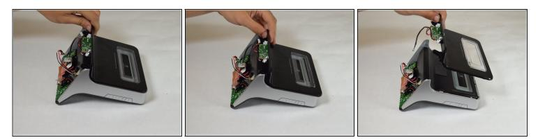
• Slide the back panel towards top of the device and lift away from the device to detach back panel.
