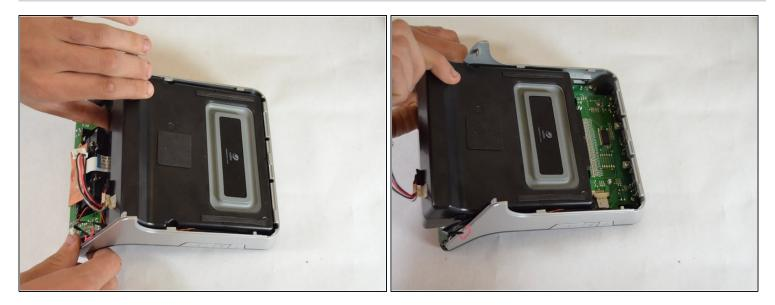
• Slide the speaker towards the bottom of the device to remove.
