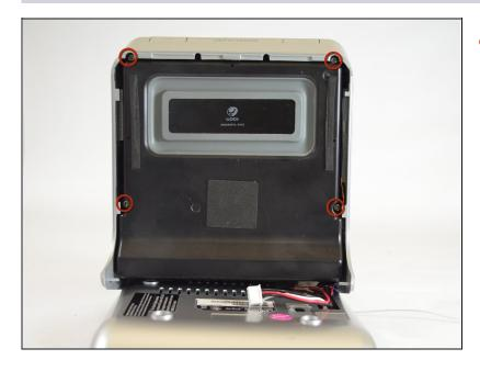
Unscrew the four 16 mm Phillips #2 screws attaching the speaker unit to device.
