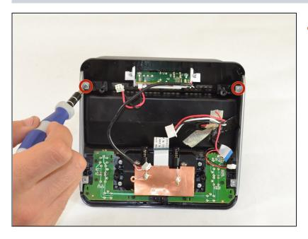
Unscrew the two 6 mm Phillips #00 screws attaching the back panel to device.
