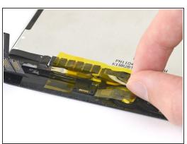
Apply polyimide tape to the area around the magnetic sensor solder pads to protect the components from heat.
