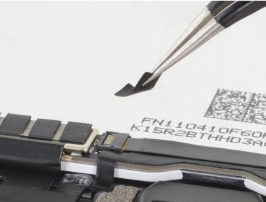
• Use a pair of tweezers to remove the sticker covering the home button assembly ZIF connector.
