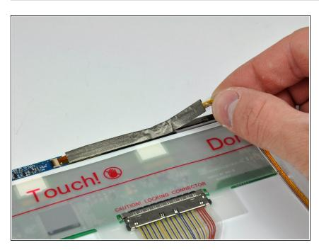
Carefully peel the camera cable off the foam tape along the top edge of the LCD.
