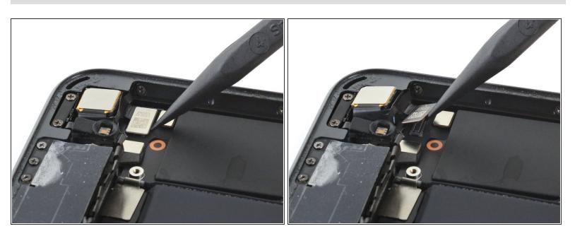
Use the pointed end of a spudger to disconnect the rear facing camera press connector.
