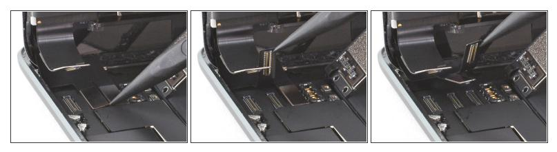
Use the pointed end of a spudger to disconnect the second and third display press connectors.
