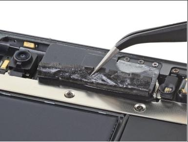
• Use a pair of tweezers to lift up the tape covering the press connector cover screws.
