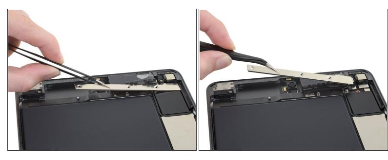
Use a pair of tweezers to remove the press connector cover.
