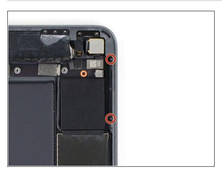
Use a Phillips screwdriver to remove the two 1.9 mm screws securing the volume control bracket.
