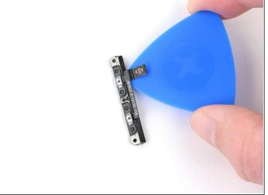
• Use an opening pick to cut through the adhesive securing the volume button cable to the bracket.
