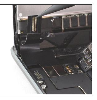
Use the pointed end of a spudger to disconnect the digitizer press connector from the logic board.
