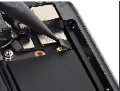
Use the pointed end of a spudger to disconnect the volume control press connector.
