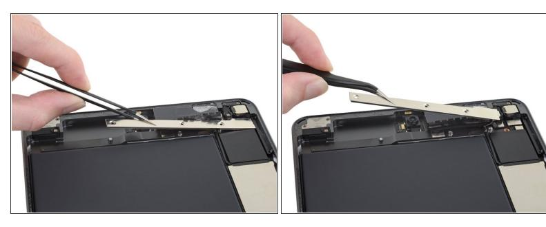
Use a pair of tweezers to remove the press connector cover.
