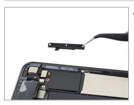
Lift and remove the volume control bracket.
