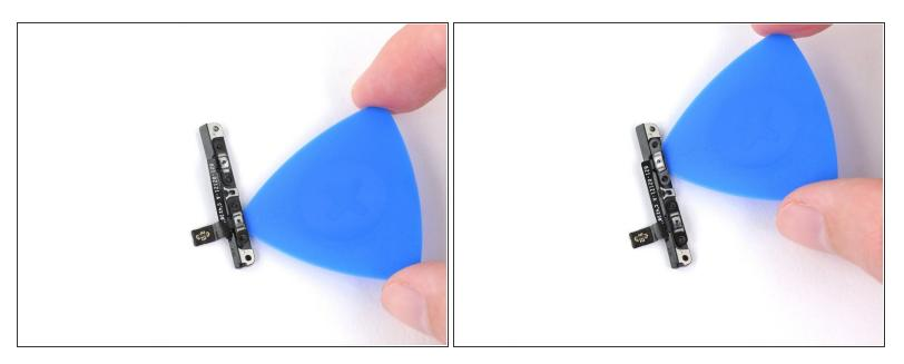
Continue to use an opening pick to cut through the adhesive securing the volume buttons to the bracket.
