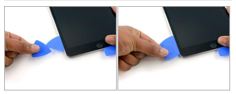
Insert a final opening pick at the lower left corner of the iPad, directly below the existing one.
