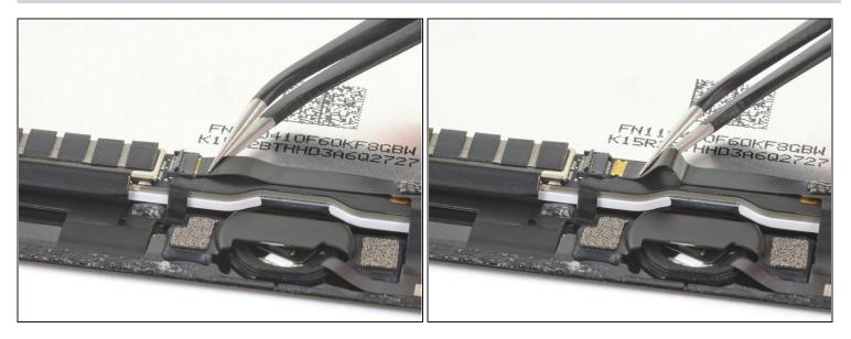
• Use a pair of tweezers to pull the home button assembly cable out of the ZIF connector.
