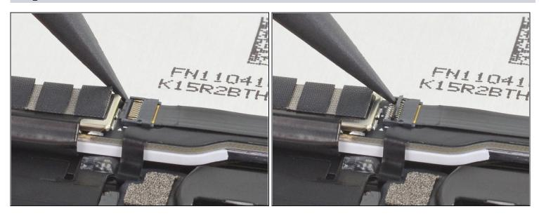
• Use the pointed end of a spudger, an opening tool, or your fingernail to flip up the small, hinged locking flap on the home button assembly <u>ZIF connector</u>.
