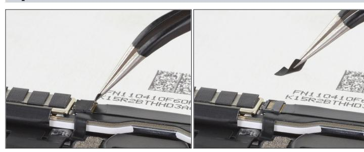
Use a pair of <u>tweezers</u> to remove the sticker covering the home button assembly ZIF connector.
