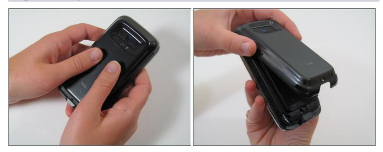
• Remove the back cover of the device by sliding it upward.
