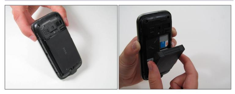
• Remove the battery by pulling it away from the back of the phone.
