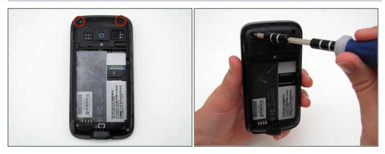
• Remove the top 2 screws on the back of the phone with the T4 Screwdriver.
