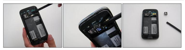
• Work the metal camera casing off by slowly prying up the sides using the spudger.
