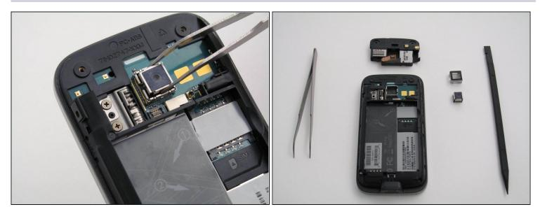
• Use the <u>tweezers</u> to pull the camera straight out of the phone.
