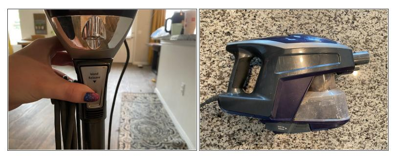
• Press the wand release button to remove the vacuum body from the roller brush and wand.
