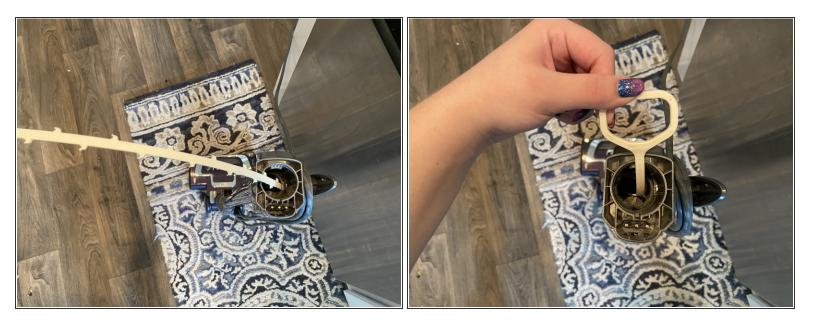
• Lastly, insert your drain snake into the tube of the vacuum to dislodge any large stuck items.
