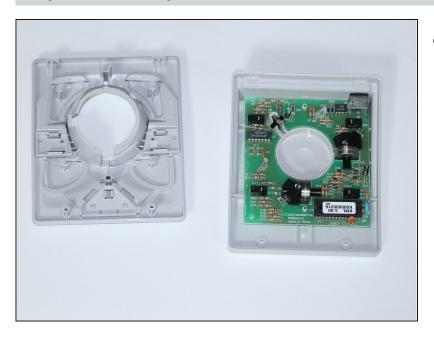
• Separate the top and bottom halves of the mouse.
