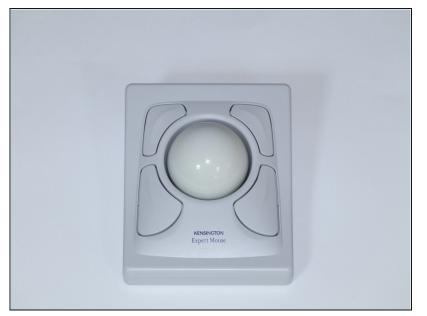
This is the Kensington Expert Trackball Mouse. This ergonomic mouse, from the 1990s, features a roller ball, and 4 tactile buttons. Begin by removing the roller ball by flipping the mouse upside down.
