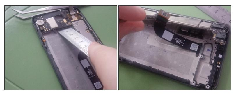
• To remove the motherboard apply adequate pressure because there will be some resistance. Try to avoid as much thermal paste as you can.
