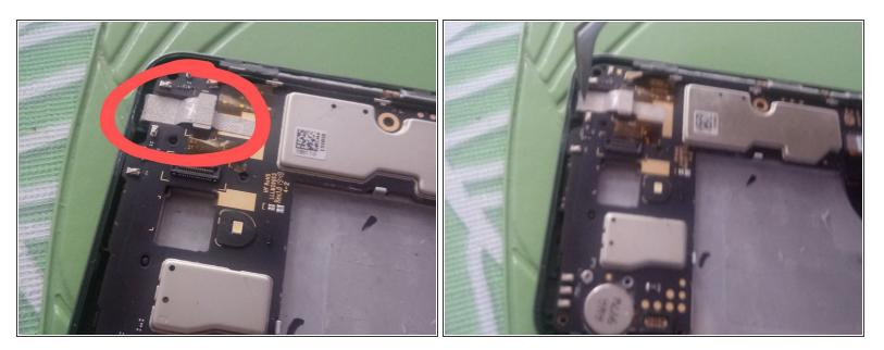
Disconnect the front camera from the phone by disconnecting the ribbon cable from the front camera attached to the motherboard.
