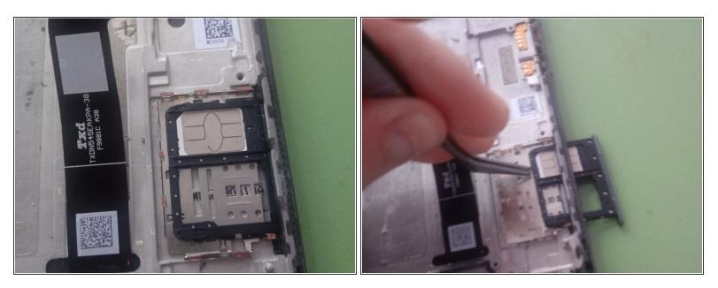
• To remove sim card just push it out the side. The sim card will be in the holder.
