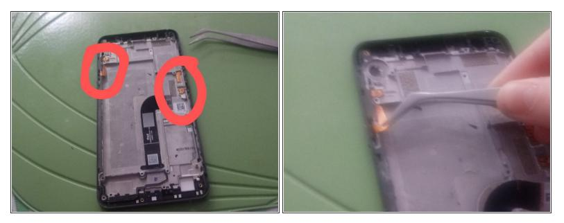
• Remove the side buttons by disconnecting the ribbon cables on each one.
