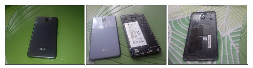
• Use a spudger to open the back panel and disconnect it from the phone.
