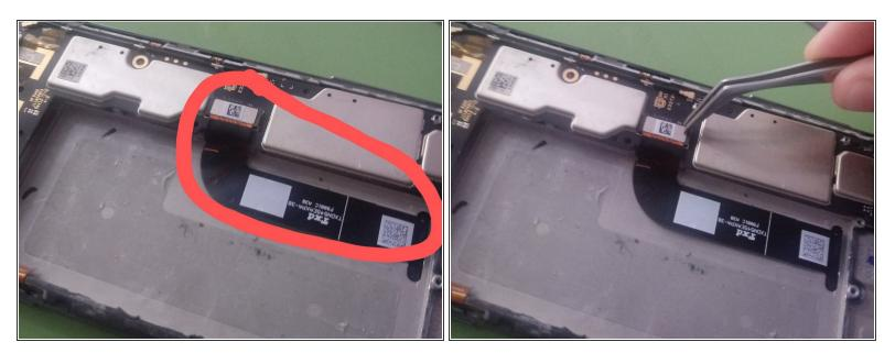
• Disconnect the display ribbon cable from the motherboard.
