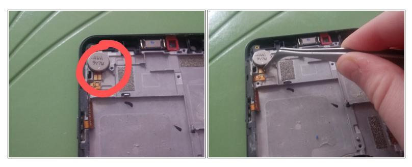
• Disconnect the ribbon cable holding down the vibrator motor then remove it.
