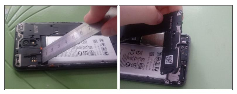
• Apply adequate force to the back panel to remove it from the phone
