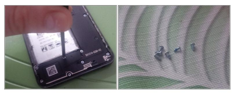
• Unscrew all 16 screws holding the back panel cover on to the phone
