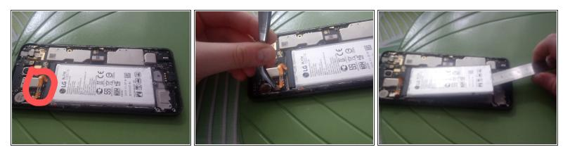
• Disconnect the ribbon cable that connects the battery to the motherboard. I suggest you heat up the battery first because of the glue and not do what i did. Use spudger to pry up the battery from the device.
