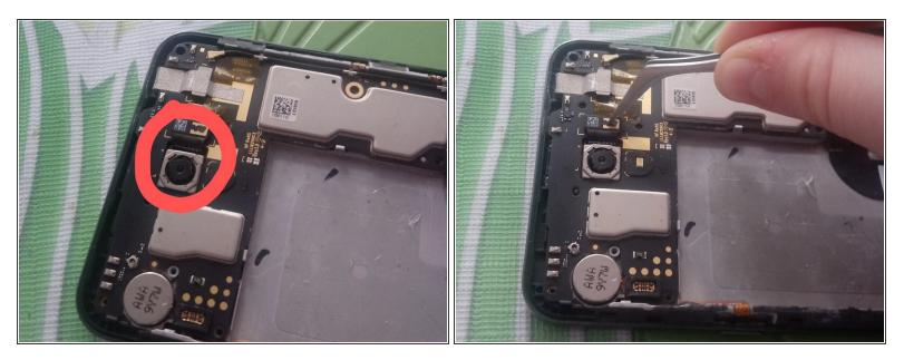
Disconnect the back camera from the motherboard by disconnecting the connector from the motherboard
