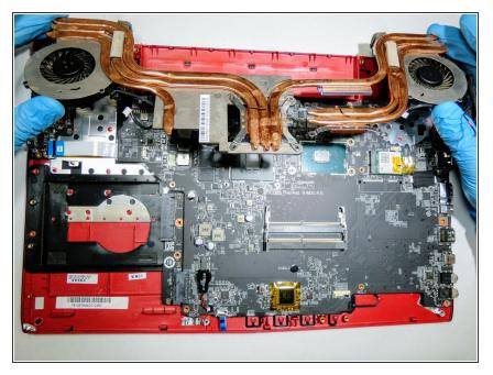
Remove the heatsink from the device.
