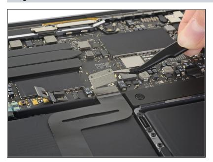
Remove the trackpad cable connector bracket.
