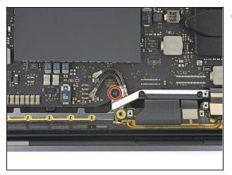
Remove the 3.7 mm T5 Torx screw securing the two antenna coax cables to the main board.
