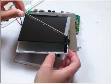
• Carefully pry the thin, metal frame from around the LCD screen.
