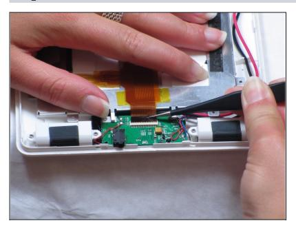
On the opposite end of the device: Remove the ribbon cable in between the speakers at the end of the battery.
