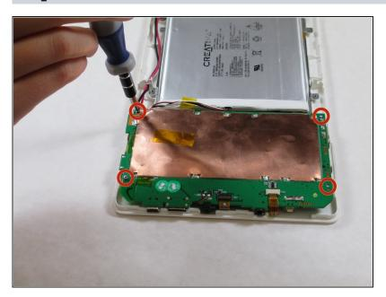
Remove the four 4mm Philips #00 screws on the edges of the circuit board.
