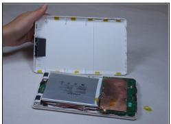
• Remove the back panel by using the plastic opening tool to carefully pry around the panel's edges.
