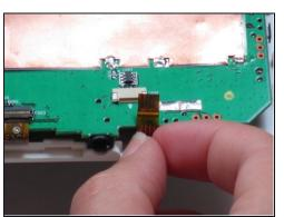
• Disconnect the ribbon cable located near the edge of the motherboard in the bottom right corner of the device.
