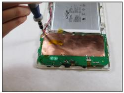
Unscrew the four Phillips #00 screws, each measuring 3mm, located at the corners of the motherboard.
