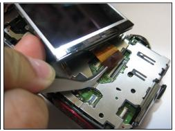
Lift LCD screen carefully from the metal casing
