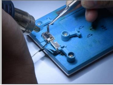
• Turn the front camera module over and attach the assembly to a holder. Heat with a hot air gun at 100 °C to remove the tape.
