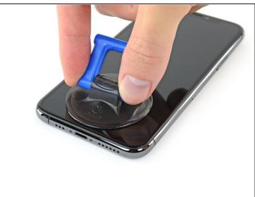
• If you're using a single suction handle, apply it to the bottom edge of the phone, while avoiding the curved portion of the glass.
