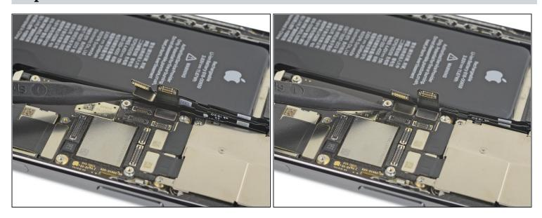
• Connect the replacement camera by pressing the connector into its socket.
