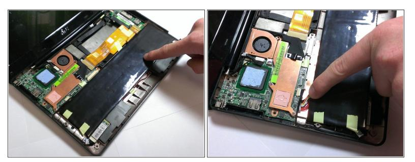
Use your fingers to lift the battery and gently disconnect the wires from the base.
