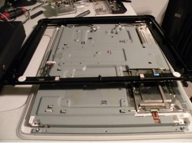
Once all of the screws are removed, lift the rim out.
