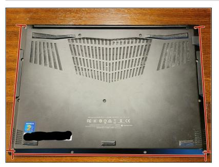
Use a plastic pick, or a very small flathead on the bottom long section, and gradually pull up the panel as you go up the sides
