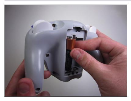
• Remove both batteries from the device.
