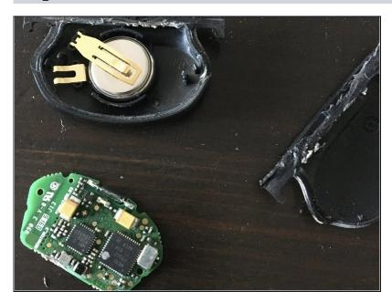
• Replacing the battery
