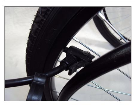
Inflate the tire to 50 psi. If there is no gauge, inflate the tire until the tire is hard.
