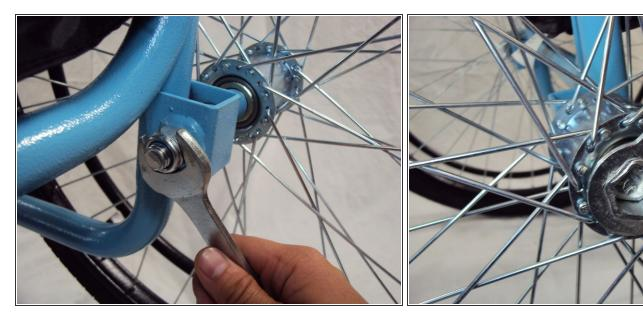
Secure the nut on the opposite side of the axle bolt and wheel. Tighten with 1/2 in or 19 mm wrench.
