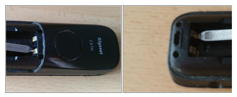
• Push in the battery contacts to be able to disassemble the housing
