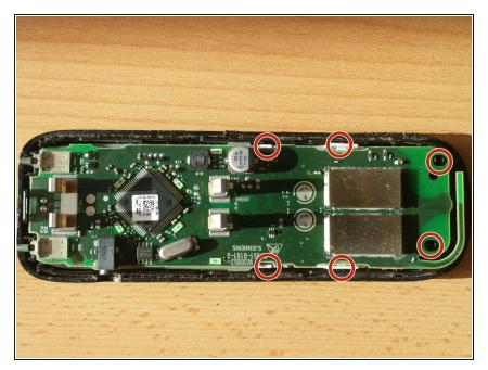
• Loosen the lugs to take out the circuit board
