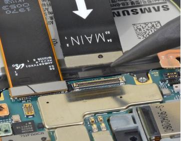
Use the pointed end of a spudger to disconnect the main interconnect cable from the motherboard.
