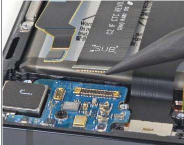
Use the pointed end of a spudger to disconnect the main interconnect cable from the daughterboard.
