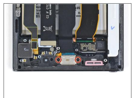
Use a Phillips screwdriver to remove the two 3.0 mm screws securing the USB-C port to the phone.
