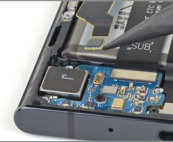
Use the pointed end of a spudger to disconnect the secondary interconnect cable from the daughterboard.
