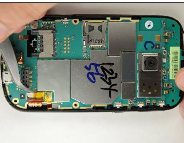
Use tweezers to carefully remove the yellow piece of tape covering the two ribbon cables.
