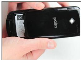
Press down on the back of the case and slide forward to remove it.
