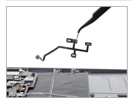
Remove the microphone array.
