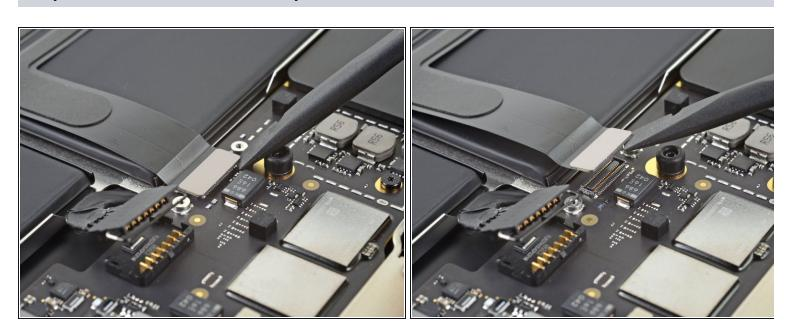
• Use the flat end of a spudger to pry the trackpad cable connector up and out of its socket.
