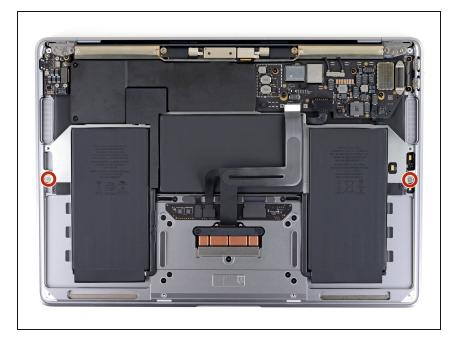
Use a T3 Torx driver to remove the two 2.6 mm screws securing the battery tray to the case.
