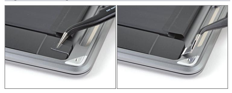
• Use a pair of <u>tweezers</u> to peel back the black pull tab on the speaker's stretch-release adhesive until you can grip it with your fingers.
