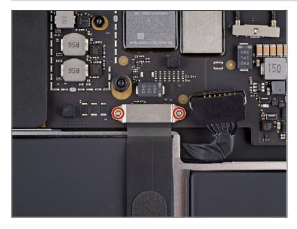
Use a T3 Torx driver to remove the two 1.4 mm screws securing the trackpad cable cover.
