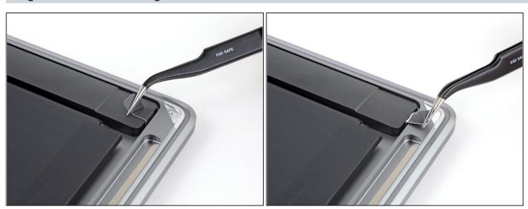
• Use a pair of <u>tweezers</u> to peel back the black pull tab on the speaker's stretch-release adhesive until you can grip it with your fingers.
