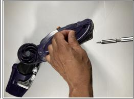
Turn the T10 Security Bit screwdriver counterclockwise to remove the 15mm screw.
