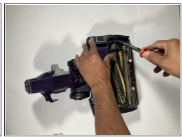
Use a spudger to pry the side of the vacuum open.
