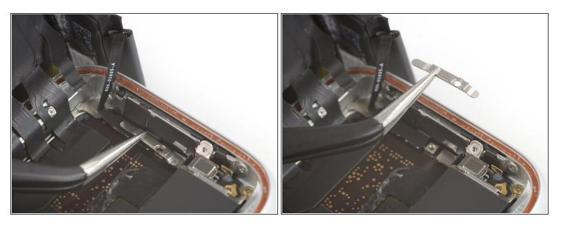
Use a pair of tweezers to remove the metal plate covering the battery connector.
