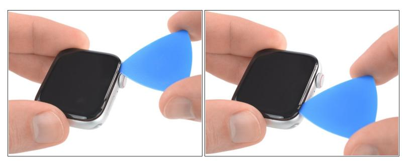
↑ When slicing near the crown, don't insert the opening pick deeper than 1/16th of an inch (~2 mm).
