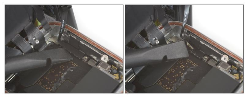
Use the flat end of a spudger to pry up and disconnect the battery flex cable.
