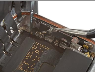
Use a pair of tweezers to carefully free the battery connector by peeling off the overlapping foil.
