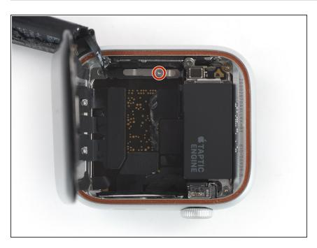
Use a Y000 driver to remove the 1.1 mm screw from the battery connector.
