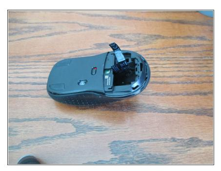
Now you can easily separate the bottom and the top of the device. (Just give it a little tug)
