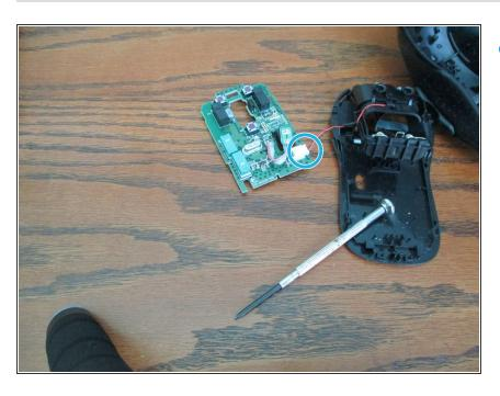
Now disconnect the cable there is circled in blue by unplugging it from the logic board.
