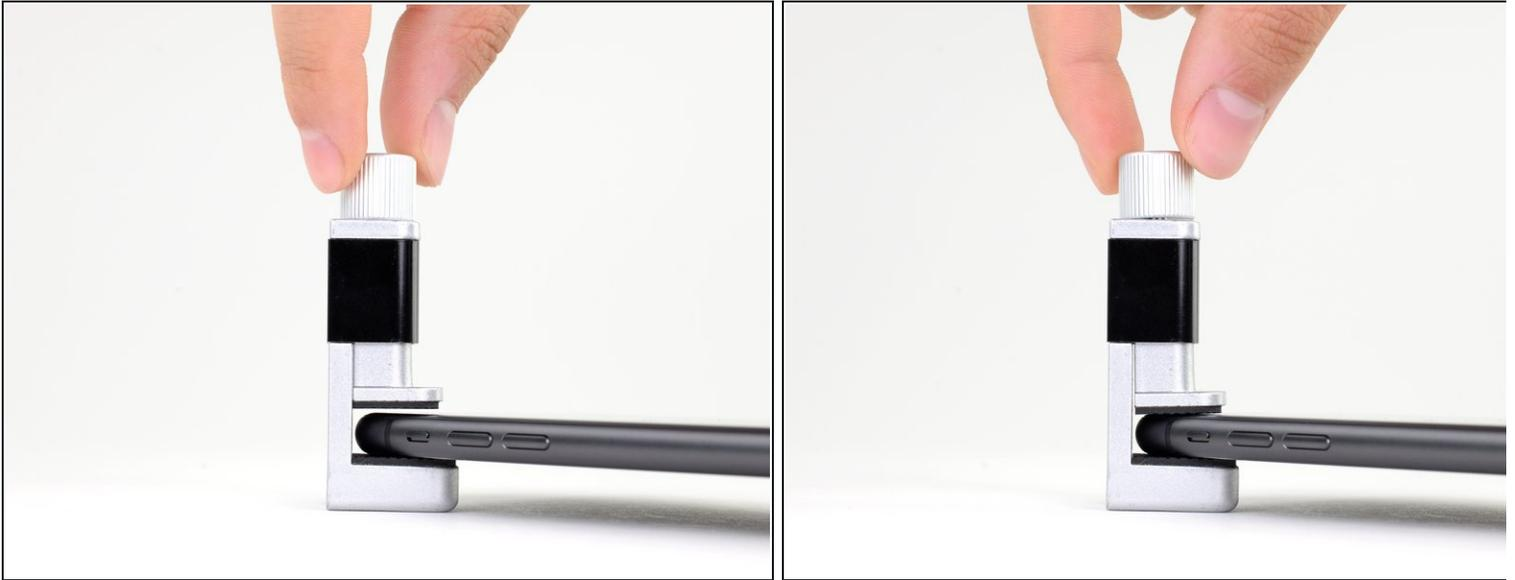
**⚠** Over-tightening may damage your device's screen or back cover.
