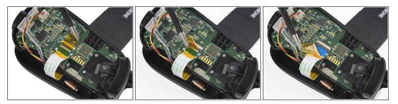
Use a pair of tweezers to remove the yellow protective tape which is placed over the interconnect cable and the connector.
