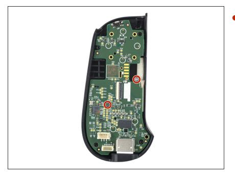
• Use a Phillips screwdriver to remove the two 3.9 mm-long screws.
