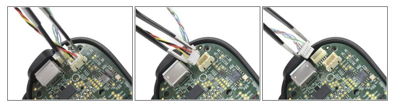
• Use a pair of tweezers to disconnect the phone connector cables out from their sockets.
