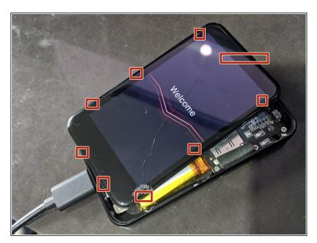
Pry the sides of the device carefully (or not if your screen is shattered).
