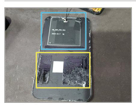
I removed the backplate, but for LCD or battery replacement is not necessary. The battery was glued to the back and there is an antenna on the top.
