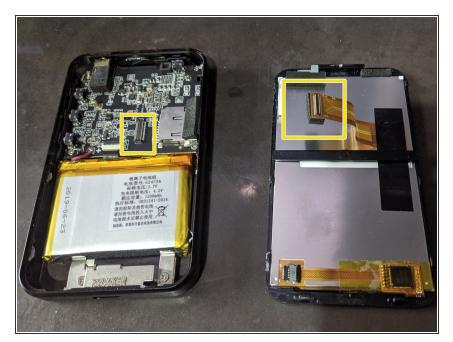
Disconnect the LCD ribbon connector in the middle of the frame and you can separate the LCD from the frame. At this point you can put a replacement LCD.
