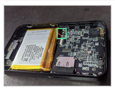
Top view of the device opened, the battery is soldered with a little of conformal coating on top of the pads.
