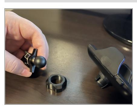
Remove the tightening knob and set the broken clip aside or toss it in the trash.
