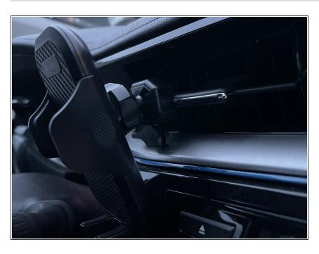
Line up the jaws with the car vent and then use the knob on the bottom to close the jaws.
