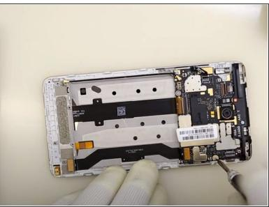
Use a Phillips #00 screwdriver to remove the eight screws fastening the motherboard to the phone's interior.
