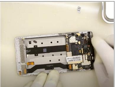
Use a pair of tweezers to remove the small metal piece from the top of the motherboard.
