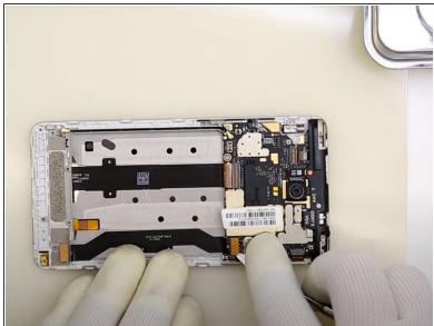
• Use a spudger to disconnect all marked ribbon cables.
