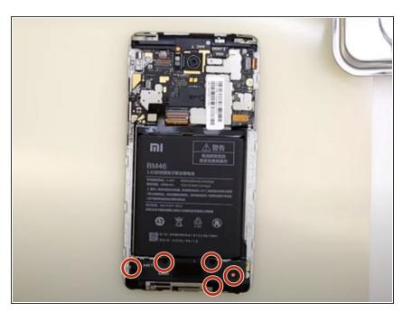
Use a Phillips screwdriver to remove the five screws in the plastic covering at the bottom of the device.
