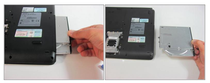
• Pull the optical drive to remove it from the computer body.
