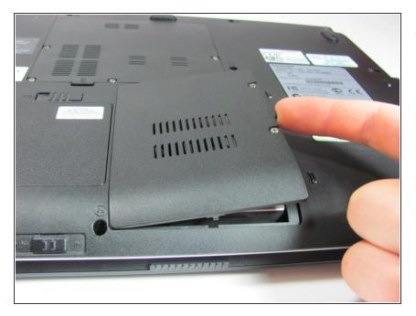
• Use a finger to lift up on the tab and remove the panel.
