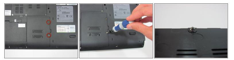
• Remove the two screws holding the hard drive panel down.
