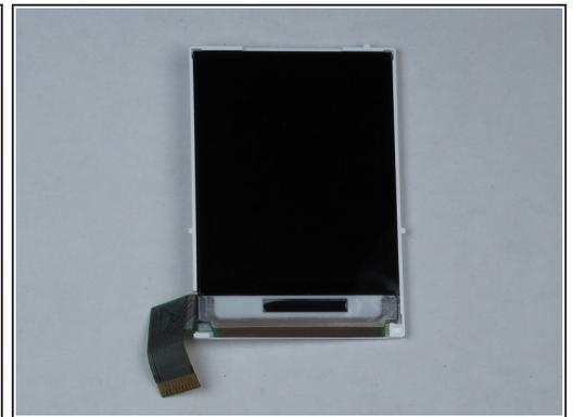
**⚠ The LCD ribbon is adhered to the memory board with a strip of glue.**
