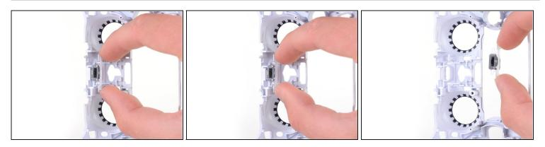
• Use your fingers to lightly pinch the plastic clip securing the microphone mute button to the front case and remove it.
