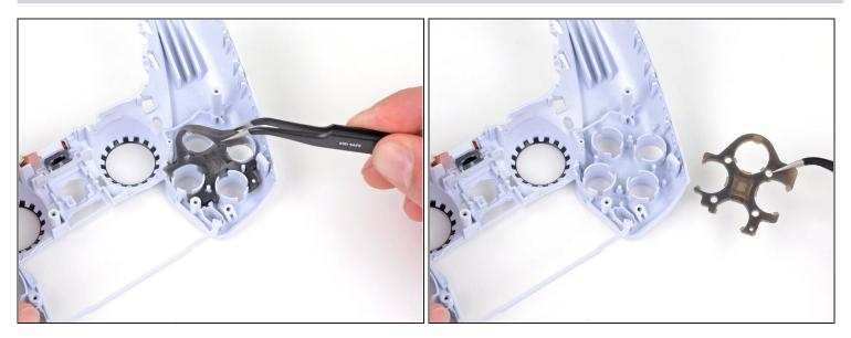
• Use a pair of tweezers or your fingers to remove the rubber insulation pad from the front case.
