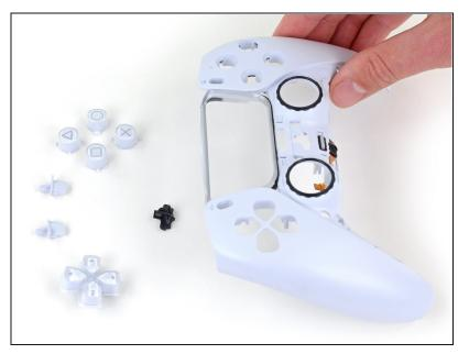
• Hold the front case close to the surface of your table and slowly turn the front case over to let the buttons fall out.
