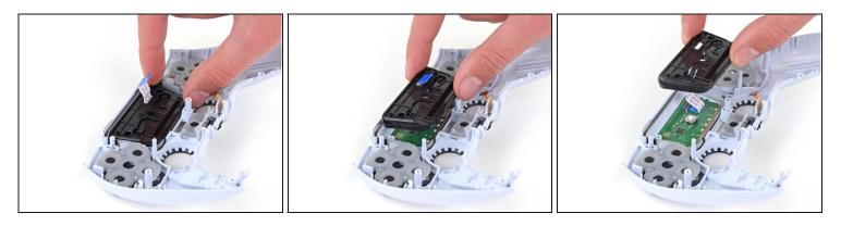
• Lift the touchpad bracket straight up off the front case.
