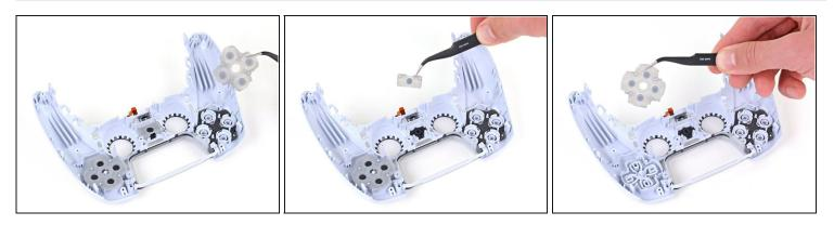
• Use a pair of tweezers or your fingers to remove the three conductive silicone rubber pads from the inside of the front case.
