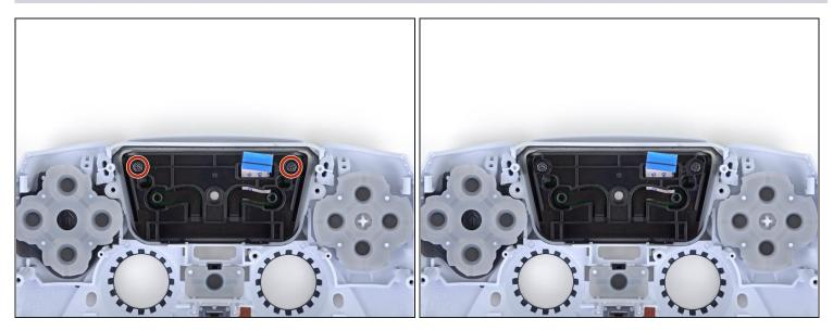
• Use a Phillips screwdriver to remove the two 6.4 mm screws securing the touchpad bracket to the touchpad.
