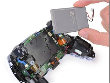
• Lift the battery straight out of the battery bracket.
