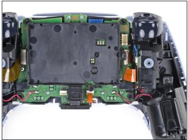
• Use a Phillips screwdriver to remove the 6.4 mm screw securing the battery bracket.
