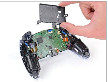
Lift the battery bracket out of the motherboard.
