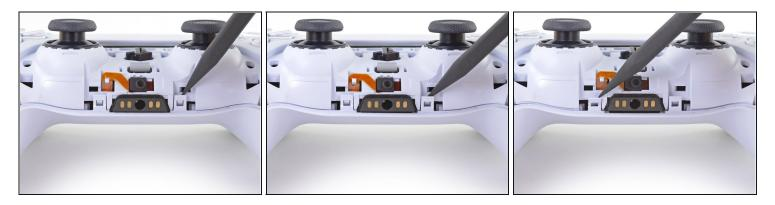
• Use the pointed edge of a spudger to unclip the two clips on either side of the headset jack.
