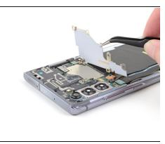
• Use a pair of tweezers to lift up and flip back the motherboard shield.
