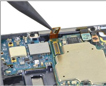
• Use the pointed end of a spudger to disconnect the touch layer cable connector from the motherboard.
