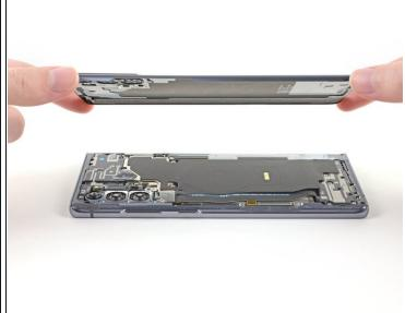
• Lift the rear cover straight up to remove it.
