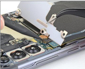
While using a pair of tweezers to hold the motherboard shield out of the way, use the pointed end of a spudger to pry up the wireless charging coil press connector.
